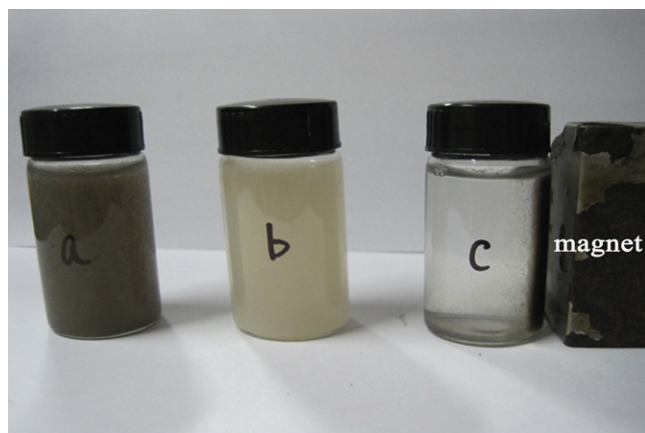
Fig. 8. Magnetic separation and immobilization of P. phragmitetus LSSE-09 cells: (a) appearance of the cell suspension immediately after adding magnetite nanoparticles; (b) free cells in Tris-HCl buffer (50 mM, pH 9.0); (c) after 2 min, the coated cells concentrated and collected by an external magnet.
